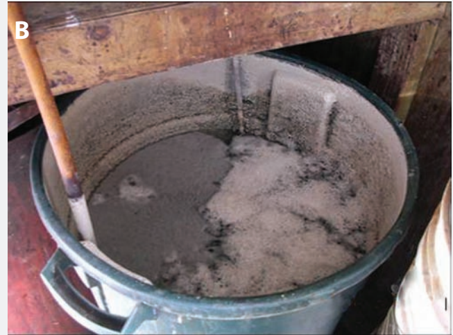
Figure 1: Water-soluble product precipitation in stock-solution containers that resulted in clogged medicator input lines. A: Container completely lined with crystals and black sludge. B: Container completely lined with white crystals, with precipitated product floating. C: White precipitate throughout the solution. D: Precipitated product floating.
