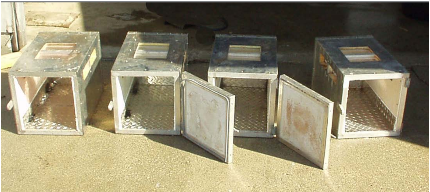
Figure 1: Four 1:150 models of full-size weaned-pig trailers were designed to allow for an equivalent animal density within the model trailer (2.5-kg pigs at 0.07 m 2 per pig) compared to a full-sized trailer loaded to capacity (300 five-kg pigs). Dimensions are provided in Table 1.
